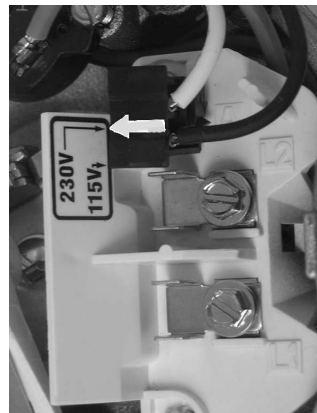
Figure 4A -Voltage Change Plug Set for 230 Volts
